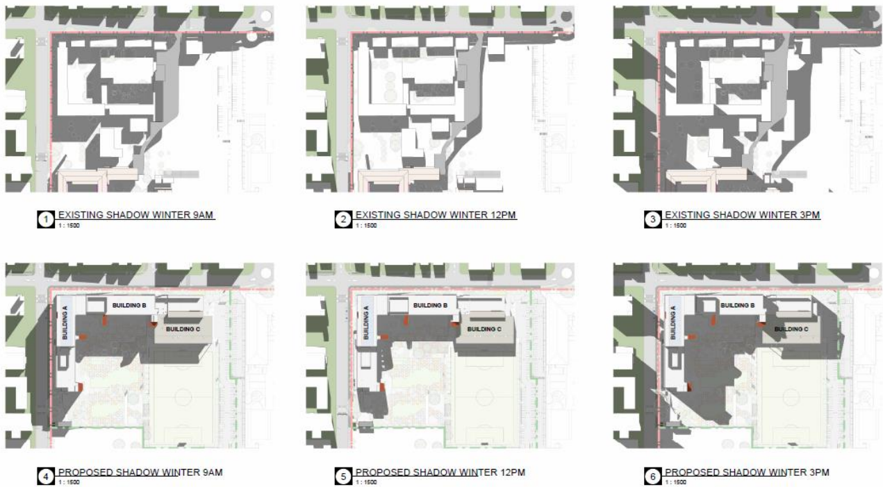
Figure 19 Existing (top) versus proposed (bottom) overshadowing impacts
