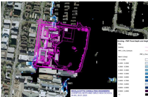
Figure 26 Existing PMF flood depth and height
